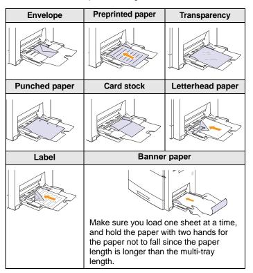
4 Squeeze the multi-purpose tray paper width guides and adjust them to the width of the paper. Do not force too much, or the paper will be bent, which will result in a paper jam or skew.
